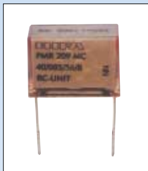
RC-Unit The RC-unit serves for limiting voltage peaks, which are produced when switching off by inductances integrated in the fluorescent lamps. It is recommended to attach with each fluorescent lamp a RC-unit. The RC-unit does not replace the conventional overvoltage protection!
